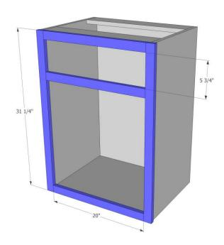
Cut the bottom trim from 1×6's. Miter the ends as shown and drill pocket hole screws at the miters. Screw the trim pieces together, then attach the assembly to the bottom of the cabinet using glue and brads.
