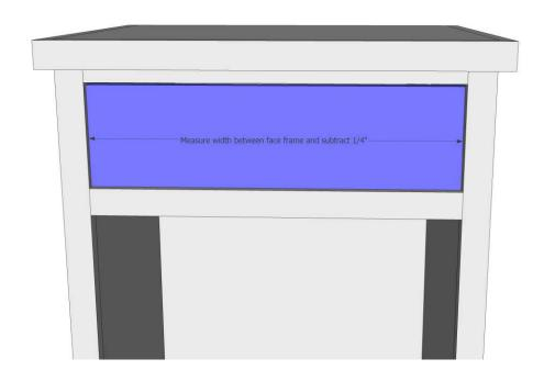
Cut the drawer front from a 1×6 board. Predrill holes in the front of the drawer box slightly larger than the diameter of the screws you will use to attach the drawer front. Adjust the drawer front so that there is an 1/8" gap all the way around and attach the drawer front to the front of the drawer box with wood screws. Double sided tape will help to hold the drawer front in place on the drawer box.
