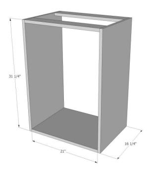
Cut the back from  $\frac{1}{4}$ " plywood and assemble using wood glue and brads.
