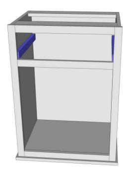
Cut the top from 3/4" plywood to the dimensions shown. Drill pocket holes on the bottom of the plywood piece at the front and side edges. Miter 1×2's to fit and attach to the top using pocket hole screws and glue.
