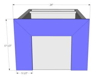
Cut drawer slider supports to fit inside the cabinet from I×2's. Align the bottoms of the drawer supports with the top of the middle horizontal rail on the face frame. Attach to the inside of the cabinet with wood screws and glue.
