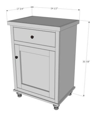
Cut the sides and bottom of the cabinet from  $\frac{3}{4}$ " plywood. Cut two I" x 4" pieces to tie the sides of the cabinet together at the top (this saves on plywood since the top will be added in a later step). Drill pocket holes in the bottom of the bottom piece, inside the front edge of the side pieces, and on the ends of the I x 4's. Drill holes for shelf pins on the insides of the cabinet sides. Assemble all the pieces using pocket hole screws and glue
